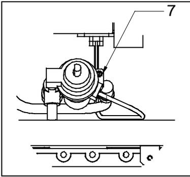
Figg. – Abb. 13 : Sostituzione del By-Pass \ Changement du by-pass \ Substituting the By-Pass \ Austausch des By-Pass \ Cambio del by-pass
